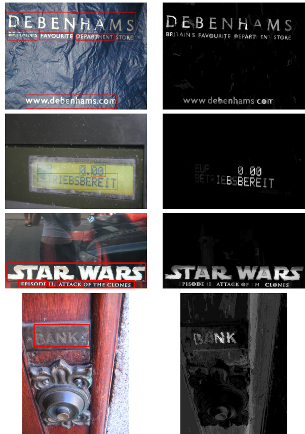
Figure 6. Some successful results from our algorithm. Left: image with superimposed detected word-level regions. Right: heat map.
