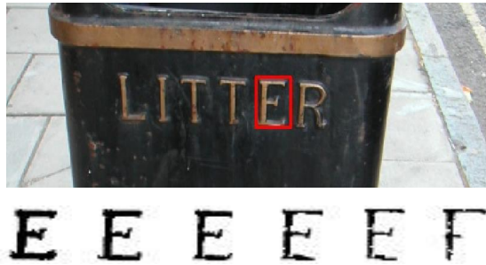
Figure 3. MSERs within a cluster centered at the red rectangle (only a few shown). The MSERs are ordered in decreasing value of fullness. The MSER to the left is chosen as the cluster representative in Stage II.
