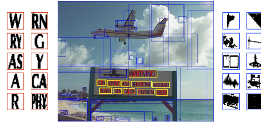
Figure 4. Mining positive (red) and negative (blue) examples from an image that was labeled at word level (yellow rectangles). Only a subset of MSERs are shown on the image for readability.
