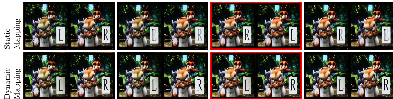
viewer at position 1 viewer at position 2 viewer at position 3 viewer at position 4 Figure 3. A static LLRLLRRR mapping of legacy 2-view content onto our 8-view display results in stereo inversion for some eye positions, with left and right images swapped. Dynamic mapping provides the correct view to each eye regardless of viewer position.
