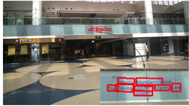
Figure 3. By cascading segmentation (TextSegNet) with detection (WordDetNet), our algorithm can detect both large and small words. If only WordDetNet is used, as trained on whole images, detection will fail in the case of too small words. Detected words by TextSegNet + WordDetNet are shown by red rectangles, the result of WordDetNet only are shown by yellow rectangles.
