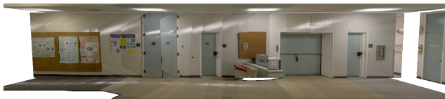
Figure 5: 3-D textured rendering of one of the walls of the reconstructed Corridor 1 scene.
